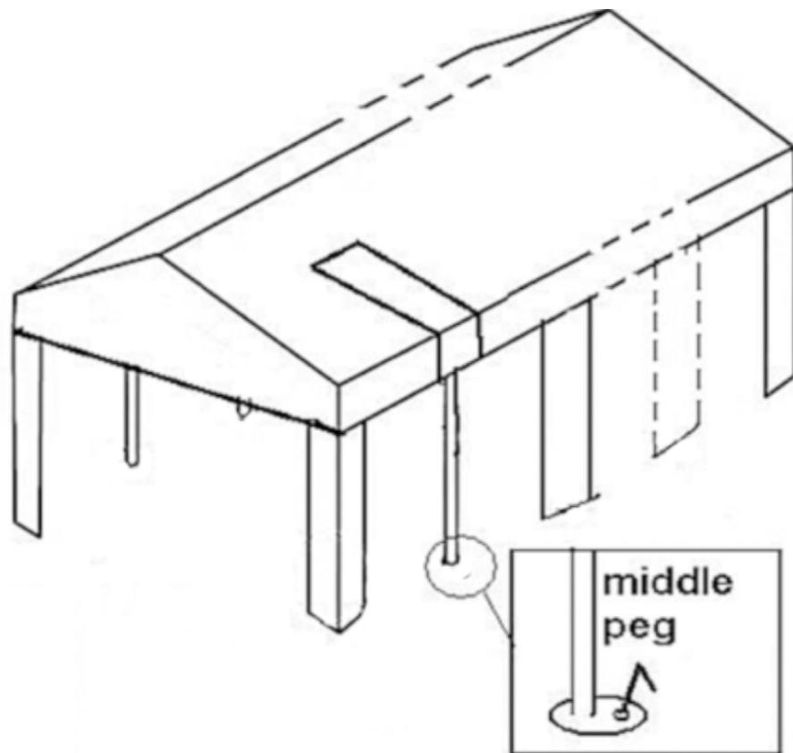
Attach the side and end walls to the framework using the bungee cords. Use one bungee cord to clasp the frame and the wall together. Use the short pegs to fix the walls to the ground.
