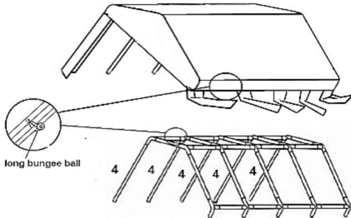
Attach the support poles (part 4) to the joints (parts 6, 7) at the other side of the tent and build up the framework. Use the long pegs to fix each pole into the ground and use the hook to fix the leg cover to the leg.
