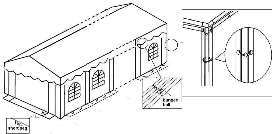
Fix the storm belts to each upper corner of the tent and fix the other end to the ground using the ground pegs.
