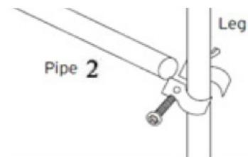
Lay all pipes and connectors on the ground and connect them to the tent frame as the picture shows. Tighten the screws afterwards.
