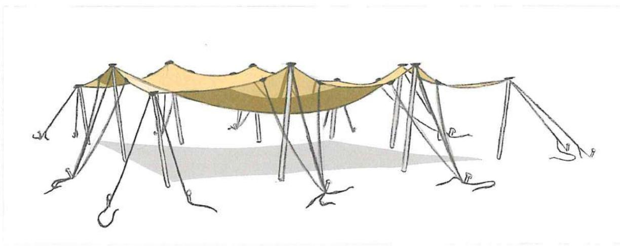
The side and corner poles are never fully perpendicular to the ground but are always slanted slightly outwards.
