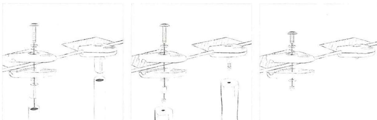
Side clamps under which an aluminium pole is standing slide easily into the pole and are fixed in place using the hand clamp.
