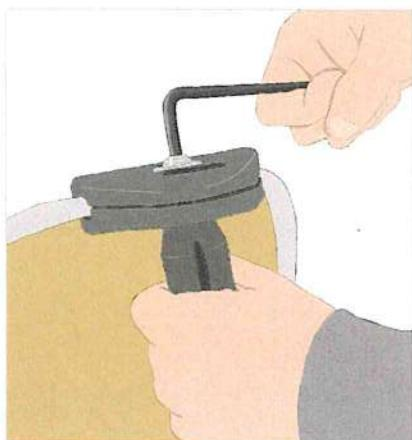
Now go to where the reinforced zones are attached on the assembly plan and fix the side clamps in the locations indicated. Always tighten the side clamps firmly. To do this you can use the hexagonal wrench supplied in the zip bag.
