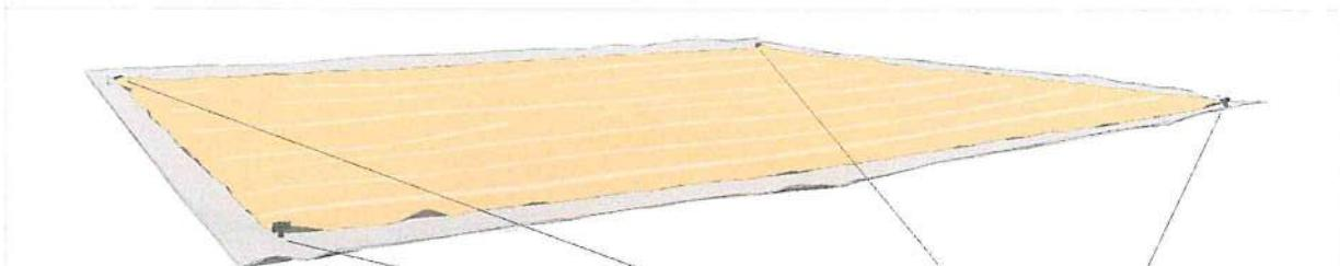
There are already 4 corner clamps attached to the corners of the stretch tent. These may not be removed or replaced. Check regularly that the corner clamp is under sufficient tension. The hand clamp of the corner clamp must always be on the underside.
