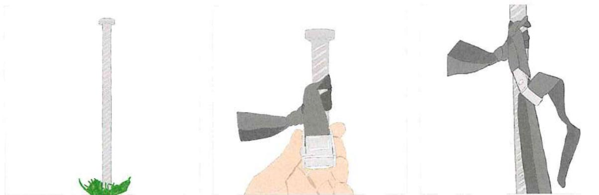
Let the tension strap lie loose on the ground for a moment and don't increase the tension on it yet. The tension straps may only be put under tension once the poles have been erected underneath the tent.
