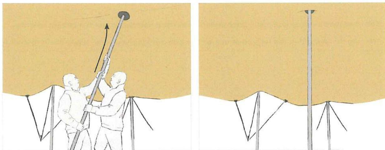
**TIP** - For tents starting from 10 x 10 m it is not easy to place the centre pole in the desired position right away. It's best to initially place one pole in a random location so that the canvas is kept floating in order for the poles to be positioned in the correct locations. The first pole that you have used as a support is then finally the last to be placed in the correct position.
