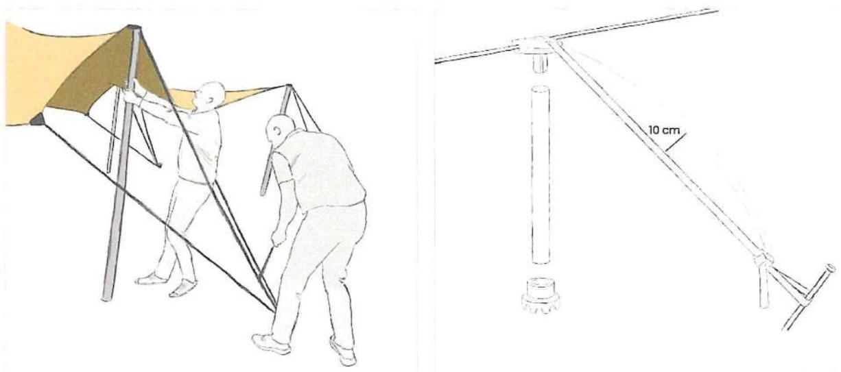
**TIP** - The tension strap can move back and forth 50 centimetres or so for the perfect tension.
