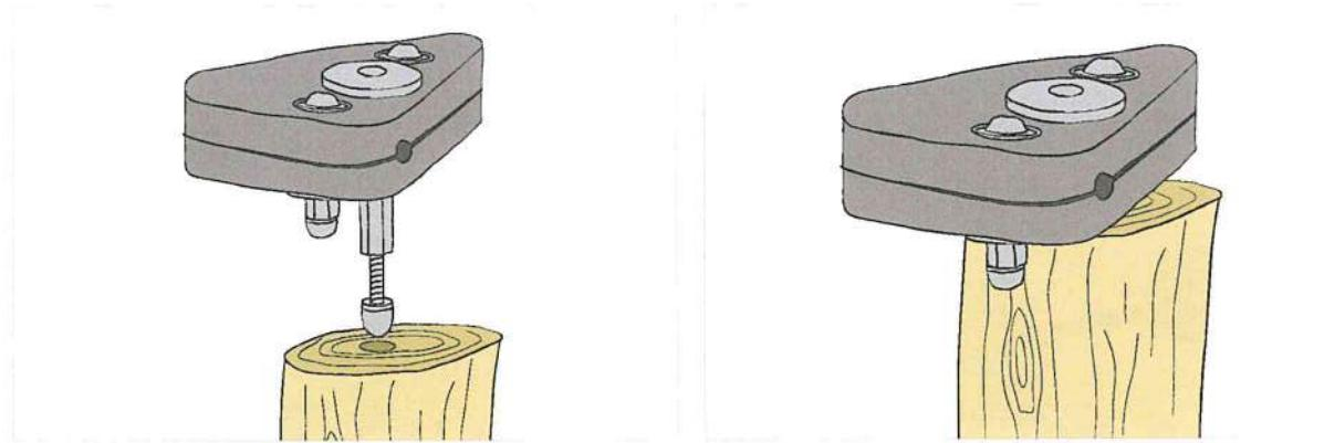
Screw the adaptor for wooden poles to the top of the centre using a screw of around 10 cm. Now slide the supplied pole caps (small or XL) over the wooden adaptor.
